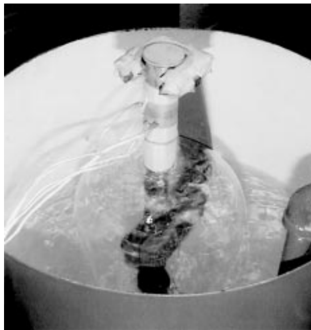
Fig. 2 Jominy end quench fixture used
